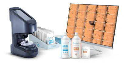
OvaCyte LA & EQ is a compact and novel point-of-care automated system that uses digital analysis and Artifical Intelligence (AI) to count and identify eggs of intestinal parasites and trematodes in a wide range of host species.
